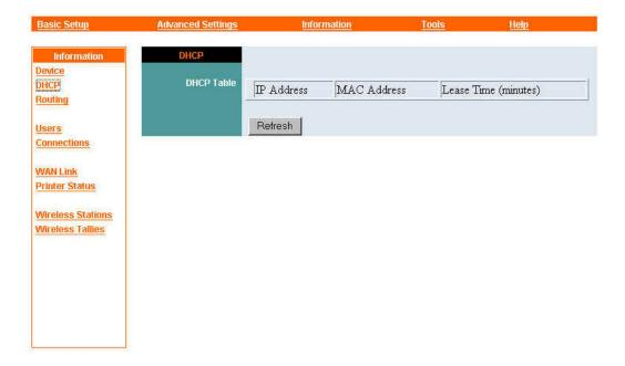
The DHCP information panel shows the IP addresses that the Wireless Gateway has assigned to machines on the LAN. Next to each IP address is the MAC address of the machine to which the address is assigned. A third column labeled "Lease Time (minutes)" shows the amount of time remaining before the machine's lease on the IP address expires. See "Advanced Settings —DHCP Server," earlier in this guide, for details.
